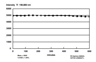
Finally, a stabilization and rinse-out test was performed with the CETAC U5000AT+. Signal stabilization (~12s) and rinse (~25s) times are both rapid as shown in the following figure.
