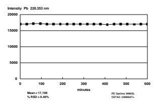
Long Term Stability Test Ultrasonic Nebulization; 1ppm Se in Drinking Water
